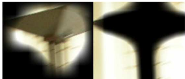
Fig. 9. Segmentation of a lamp in the home sequence. Left: Using the saliency-based segmentation algorithm. Right: Using the color-based segmentation algorithm. The color-based segmentation totally fails because in this case it uses the background pixels to set its color model.
